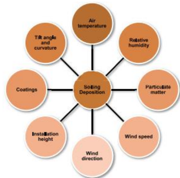
Figure 1: Factors determining soiling in solar panels (Conceição, et al. 2022).
